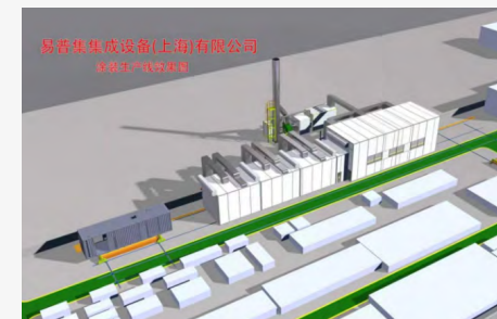
▲ Rendering of the air emissions treatment system for automated coating lines
